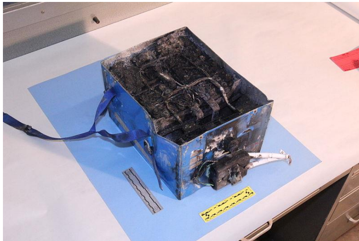
Above: Photo of the burned APU battery unit from JAL Boeing 787
