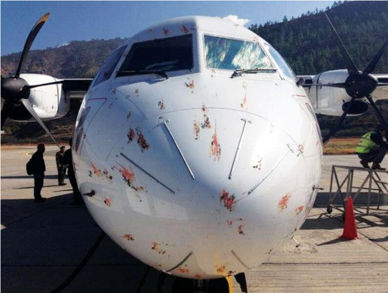
Above: Photo of an ATR-42 clearly showing bird strike residue
