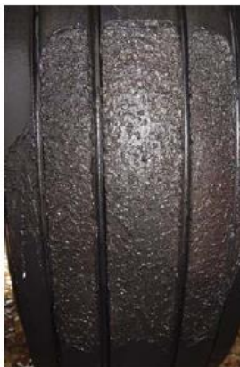
Above: figure 1 - marks of rubber reversion hydroplaning on the tyre
