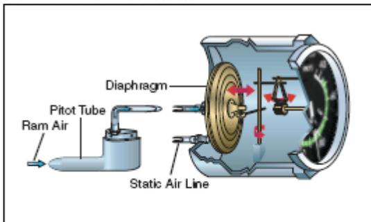
Ram air pressure from the pitot tube is directed to a diaphragm inside the airspeed indicator. The airtight case is vented to the static port. As the diaphragm expands or contracts, a mechanical linkage moves the needle on the face of the indicator.
